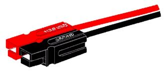
Housings should be mated according to the diagram above, viewing from the contact side (opposite the wire side), tongue (contact) down, and hood up, RED on the LEFT, BLACK on the RIGHT. The use a roll pin is not recommended as they can fall out and short a battery or power supply. In most cases the dove tailing of the connector will hold it together, if needed, a drop of super-glue will keep the housings from sliding apart.
